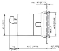
With front bezel 60 x 75 [2.36 x 2.95], panel cut-out 50 x 50 [1.97 x 1.97]
