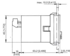
With front bezel 55 x 55 [2.17 x 2.17], panel cut-out 50 x 50 [1.97 x 1.97]
