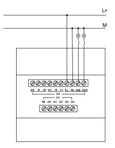
3.3 Connecting the IOT2000, Input/Output Module
