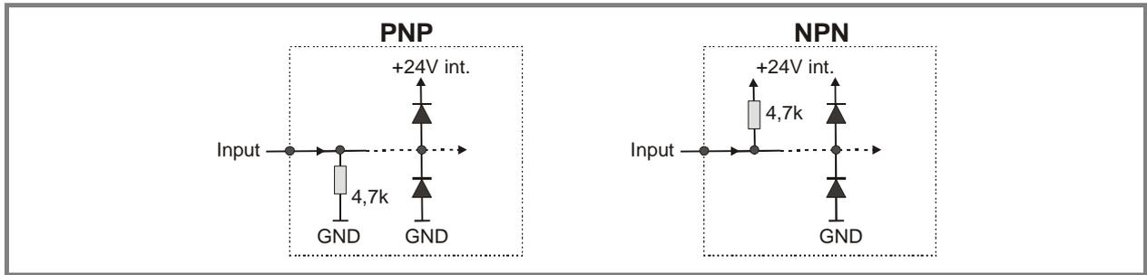
Counting inputs A and B are designed for input frequencies up to 100 KHz with all counter modes, and up to 25 kHz with all other operating modes.
