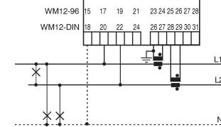
**WARNING:** the current inputs can be connected to the lines ONLY through current transformers. The direct connection is not allowed.
