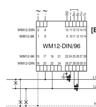
**F**- RS485 4-wire connection (the CT's must be connected to ground).
