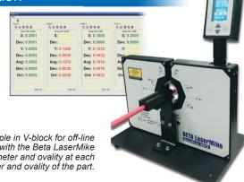
AccuScan 6012 shown with medical tube sample in V-block for off-line sample/part inspection. It can be used with the Beta LaserMike AccuNet software to display the diameter and ovality at each location, as well as the overall diameter and ovality of the part.
