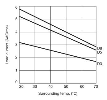
Derating curve is used for finding max. load current at an elevated ambient temperature. The 3 lines in the graph represent the 3 nominal current ratings of the RP1 series (RP1...D3/D5/D6).
