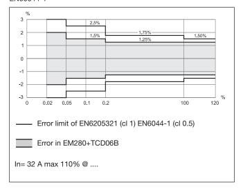
kWh, PF=0.5L, compared with a cl 1 meter EN62053-23 plus a cl 0.5 CT EN60044-1
