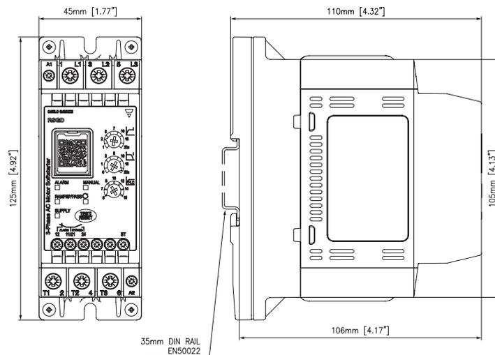
Fig. 1 RSGD..12..VD200 to RSGD..32..VD200, RSGD..12..VD210 to RSGD..16..VD210
